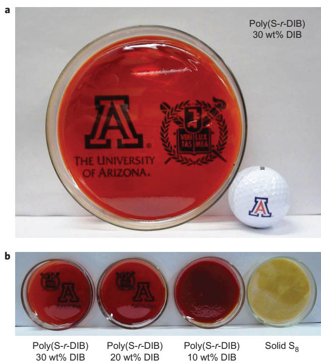
Figure 3 | Transparent glass films of poly(S- r -DIB). a , Synthesis on a 25 g scale of poly(S- r -DIB) copolymer transparent glass film with 30 wt% DIB cured in a petri dish (outer diameter, 15 cm) with a golf ball as a reference for scale (diameter, 4 cm). b , Range of compositions (from the left), 30 wt%, 20 wt%, 10 wt% DIB and elemental sulfur cured in petri dishes (outer diameter, 5 cm). The inverse vulcanization enables facile modification of the composition and properties of poly(S- r -DIB) copolymers by controlling the feed ratio of DIB used in the polymerization. The introduction of higher contents of DIB in the final copolymer enabled the fabrication of red transparent bulk films that suppressed the crystallization processes typically observed in bulk forms of S 8 .
